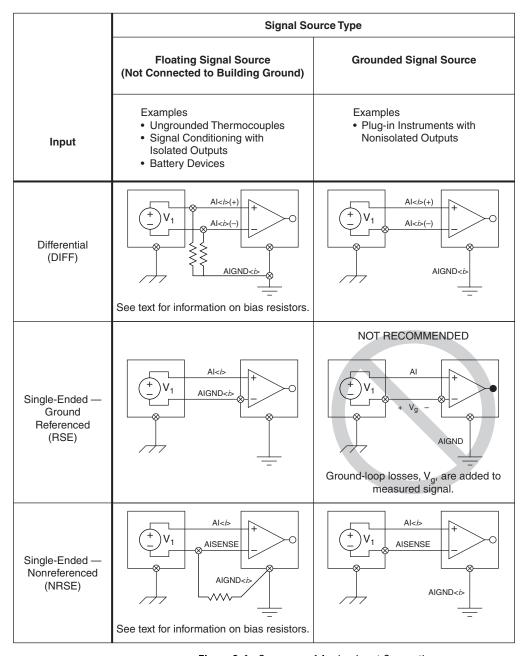
Figure 2-4. Summary of Analog Input Connections
